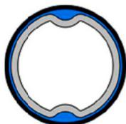
The air (in blue color) flows easily through the grooves, considerably reducing the load losses.
