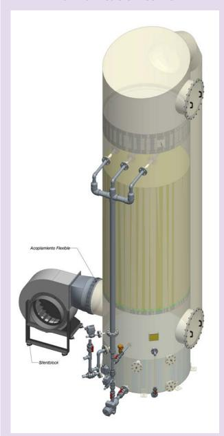
The gas flow, driven by the fan, passes through a layer of absorbent filler (Pall rings), receives a rain of water through the diffusers, to reach a droplet separator. The gas, already humidified, crosses a large pipe to the biomass bed.
