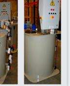
The emulsion polyelectrolyte is extracted from its storage drum by means of the **pump** which injects it, in the desired ratio, into the dilution water manifold.
